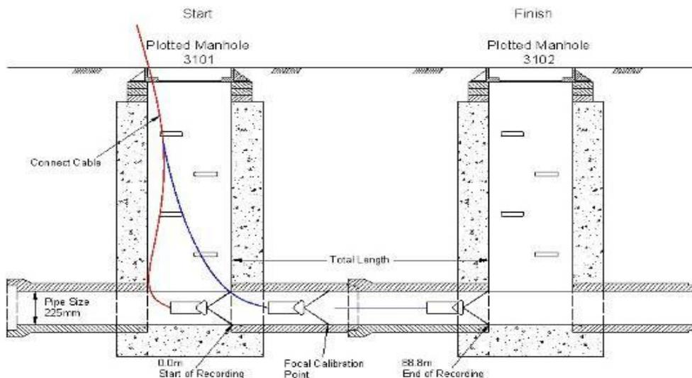
Fig. 4.2 Chainage recorded during inspection (From Manhole View)
