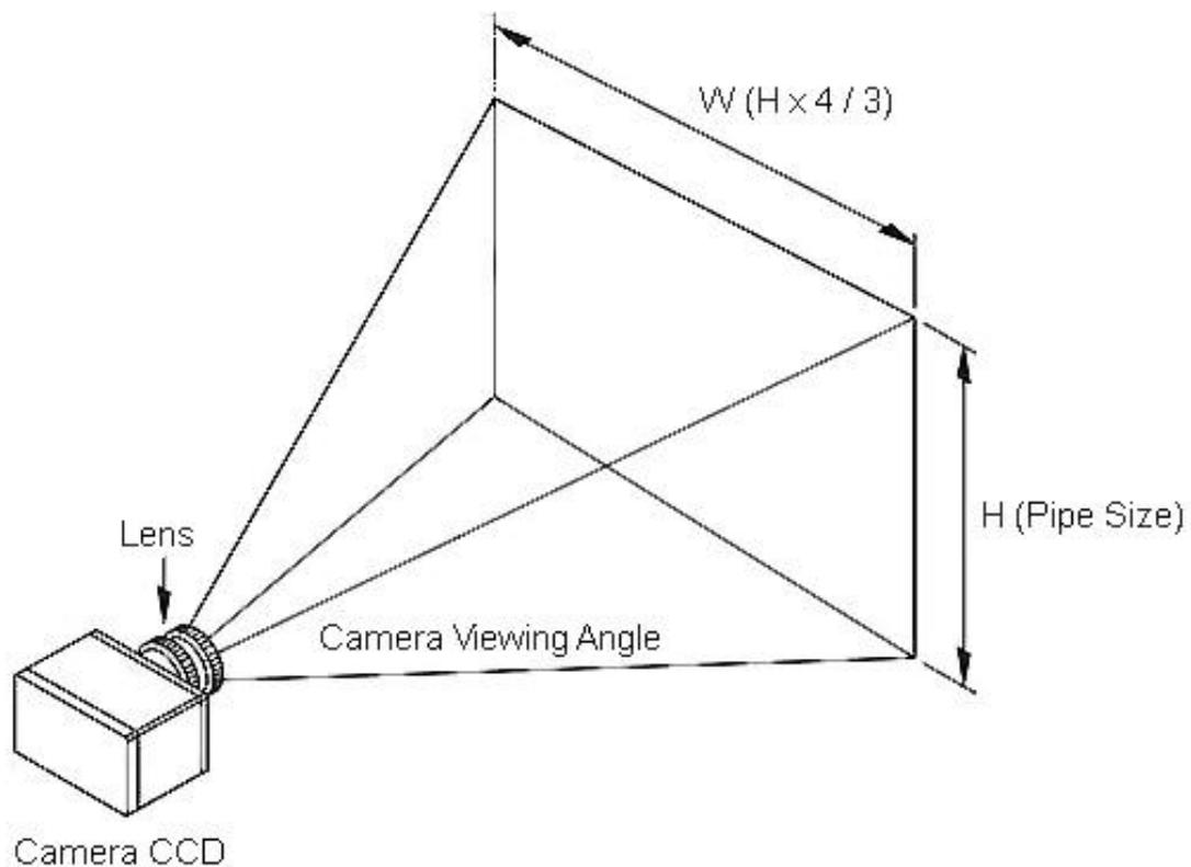
Fig. 4.4 Measurement of focal length
