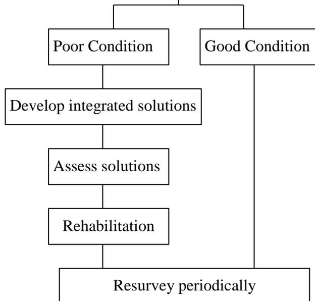
Fig. 5.3 Flow chart of conducting CCTV Survey and the follow-up actions.
