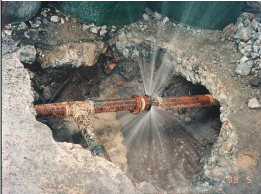
A: Water burst from a deteriorated water main.
